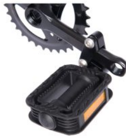
Reductor bieles pedals ajustable tricycle Momo
